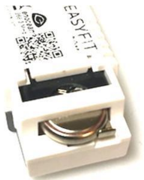
Figure 13 – Properly inserted backup battery
