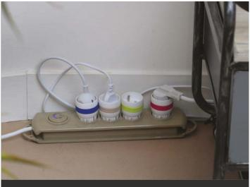
Automatically cut the power supply of multimedia devices at night\*
